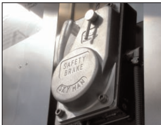
Overspeed safety brake inside cage. Pulling handle provides emergency descent at controlled speed in case of power failure.
