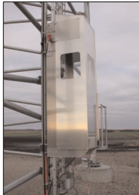
Pro-Bel TH250-U Tower Hoist Personnel Cage used in exterior application. Note cover on top to protect electrical components and power conductor rail instead of trailing supply cable.
